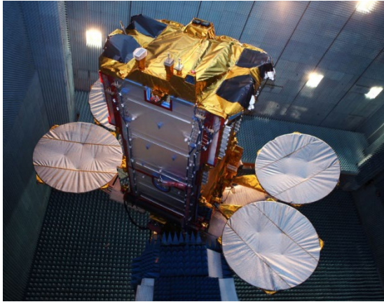
Ka-SAT undergoing electromagnetic testing in Astrium facilities
